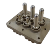
Ground power receptacle
