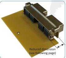
Amphenol Air LB has developped shortened SIM specific receptacles for SIM OPLF modules, thus optimizing the overall size on the PCB.
